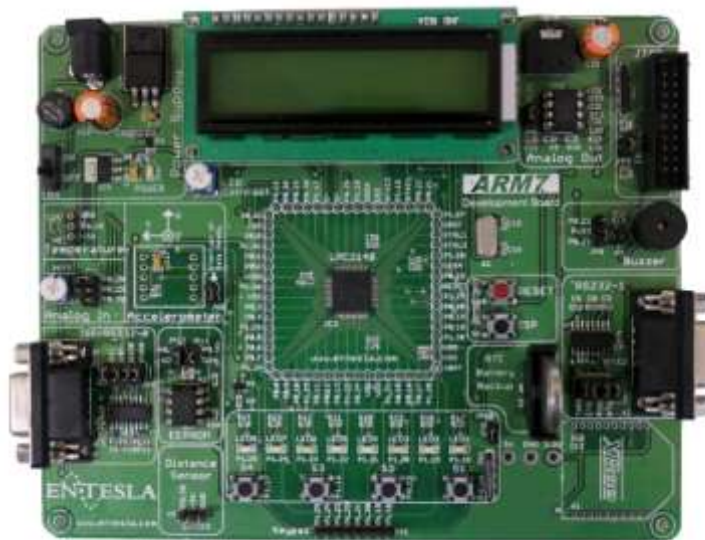
FIGURE:3 ARM 7 DEVELOPMENT BOARD
